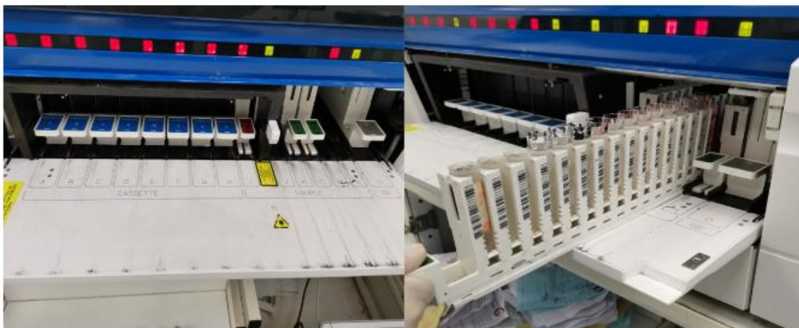
Figure-4 Inserting racks containing numbered sample cups into the device.
